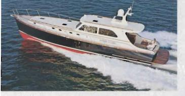
display this time around. It features 4 staterooms, 4.5 heads, a 174 sq. ft. cockpit with an observation mezzanine and a climate controlled bridge. Powered by a pair of Caterpillar C32 engines rated at 1925-hp each, the boat cruises at 35 knots and has a WOT of 40 knots.
